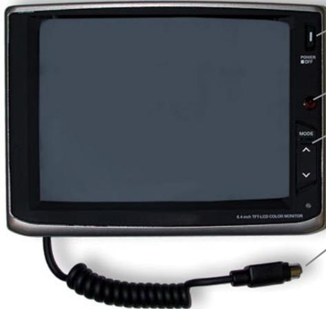
**Power button** - Press the button once to turn on the LCD. Press and hold for 1-2 seconds to power off the LCD.
