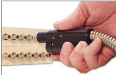
**Step 4 For bulkhead applications: Plug** the cleaning tip into the bulkhead mating sleeve as if you would, using a Westover Scientific Video Inspection Probe. Apply slight pressure against the mating sleeve and gently slide and hold the handset forward. Notice the POWER/READY LED turns green. Press the RUN
