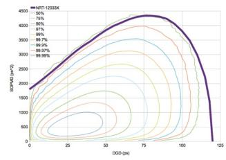
The NRT-12033X covers 99.99% of the states occurring in a 36 ps mean PMD fiber span. To the left, the joint probability density function of a 36 ps fiber is shown by the rainbow colored contours. The NRT-12033X can access all states below the dark blue curve, beyond the outmost contour. This wide DGD/SOPMD range, combined with the broad 33 GHz free spectral range enables the NRT-12033X to test, compare, design and deploy 10G/s and new generation <sup>125</sup> 40G DP-QPSK transponders.
